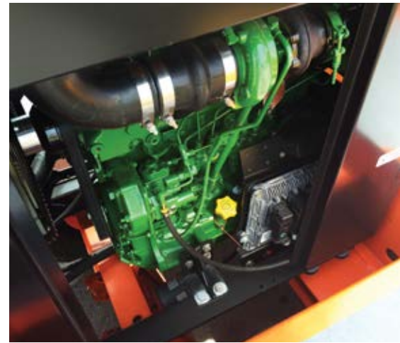
A 74-hp (55-kW) PowerTech EWX 4.5L Final Tier 4 engine supplies hydraulic power to the new SPF-8 road widener.
