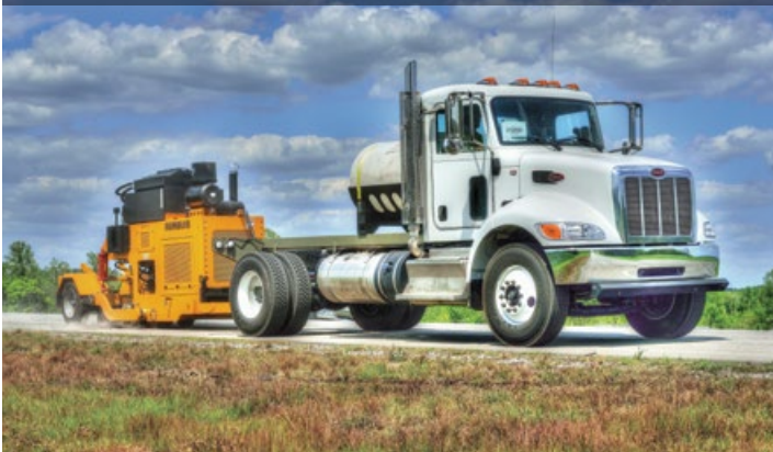
Hydraulically driven by a PowerTech 6.8L engine, the Road Pro 6200HD can be fitted with flail bits, milling cutters, diamond blades, brushes, or shot-blasting head.
