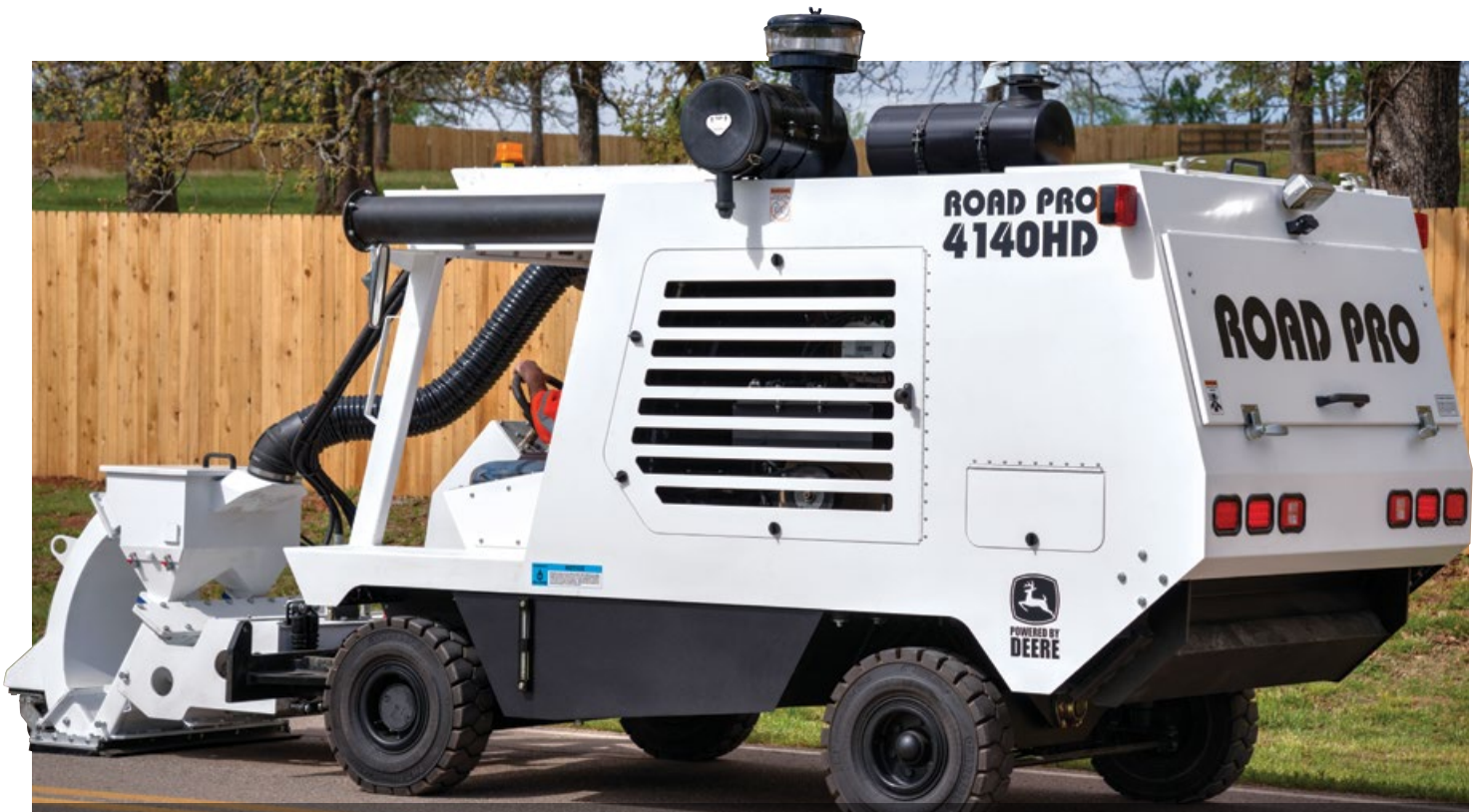
To make the RP4140HD more compact and highly maneuverable, Dickson rotated the PowerTech 4.5L engine 90 degrees to shorten the wheelbase.
