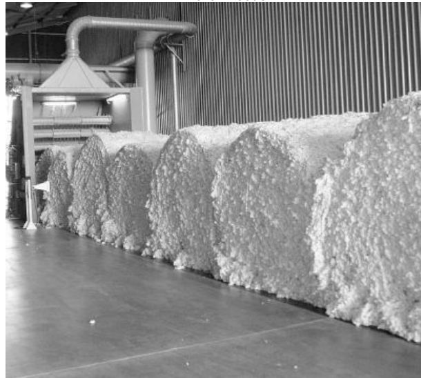
Modules Placed Perpendicular to Feed Direction
