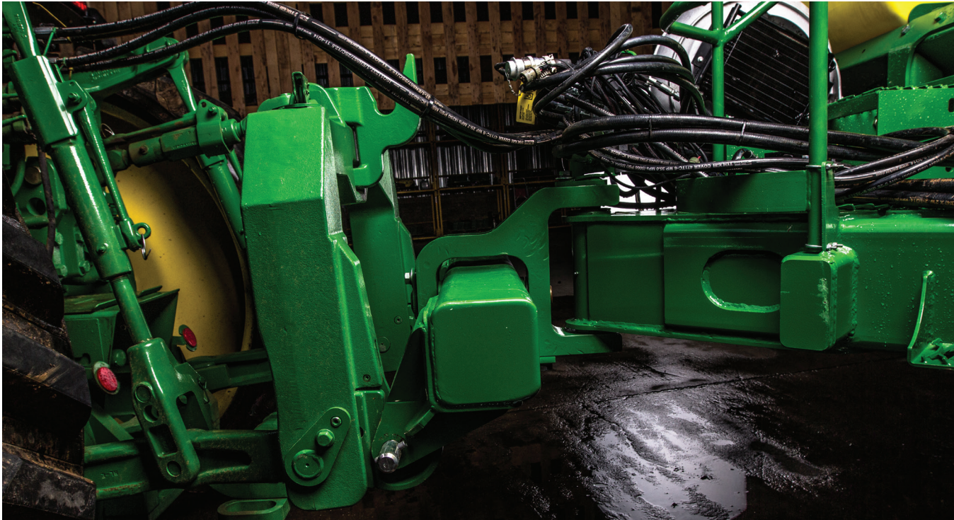
Above: Two Point hitch frame makes the correct adjustment and planting unit position easy. Two Point design for reduced transport length to get through corners.
