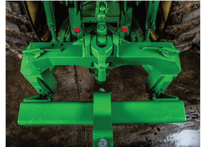
Above: Two Point hitch frame makes the correct adjustment and planting unit position easy. Two Point design for reduced transport length to get through corners.
