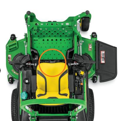
Adjustable suspension seat A fully adjustable suspension seat option features lumbar support, control dial for easy adjustment, and seat latch for easy seat lifting.
