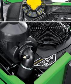
Available Electronic Fuel Injection gives you the option of turning your commercial-grade mower into a fuel-sipping dynamo. The closed-loop system allows just the right amount of fuel and spark to the engine, at just the right time – not only delivering fuel savings, but optimizing power, performance and efficiency across all mowing conditions as well. Choose from the Z925M EFI, Z945M EFI, or Z955M EFI models.
