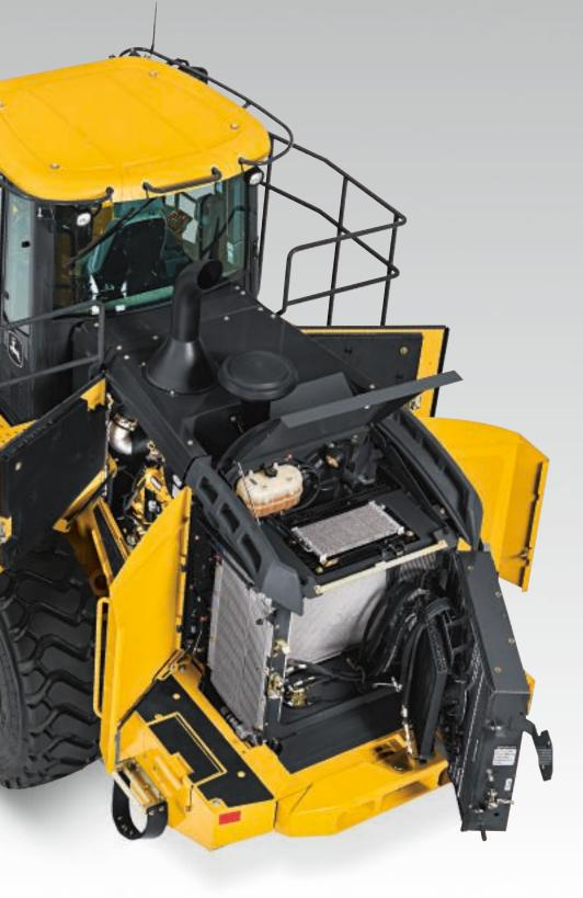
Greasing is less messy thanks to centralized lube banks that provide easy access to zerks. Conveniently located periodic lube and maintenance chart confirms that nothing gets overlooked.
