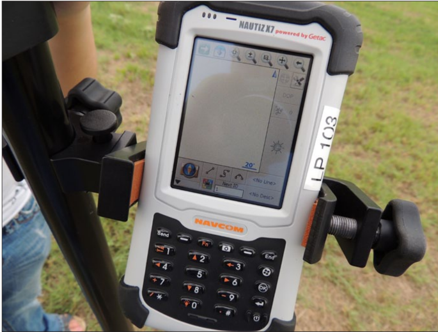
The Nautiz X7 is a rugged controller included in the LAND-PAK system and is loaded with MicroSurvey's very mature and capable Field Genius Software.
