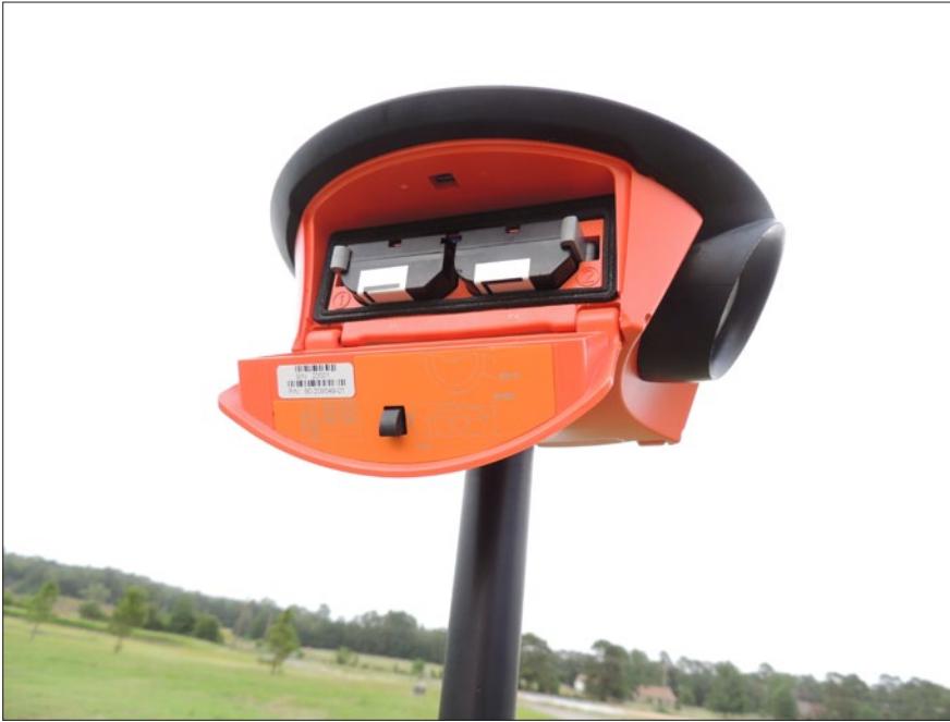
LAND-PAK base and rover are powered by two removable, hot-swappable batteries. The LED display indicates which battery is in use. The hard rubber bumper encircling the solid cased receiver gives a definite feel of durability should the unit fall over.
