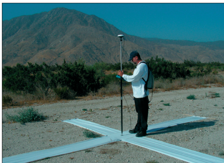
The SPEC team used the StarFire system to pinpoint and to set the location of about 300 aerial survey control panels.
