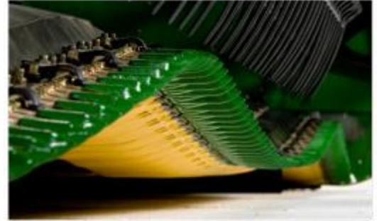
**HD:** With the wings in the down, measure 45mm at the outer reel fingers and 15mm at hinge.
