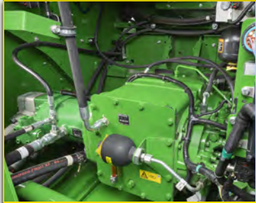
A. Clean transmission, hydraulic valve block, and front axle area.
