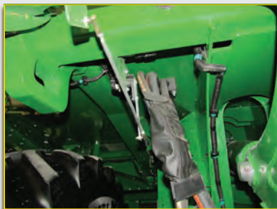
A. Clean and check the handler position sensor.
