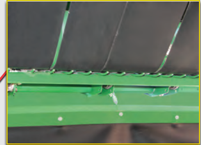
C. Clean and check the wrap feed rods. Clean out the debris around the lower gate roller.
