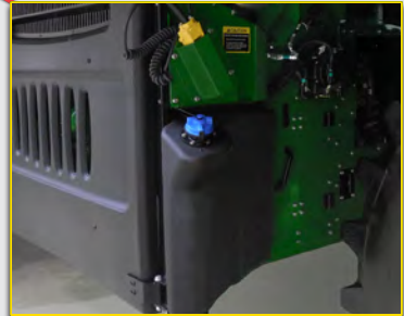
F. Clean the diesel exhaust fluid (DEF) tank and pump (if equipped). Clean access panel latches.
