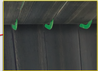
D. Lower the rockshaft and operate the belts to check the tracking.
