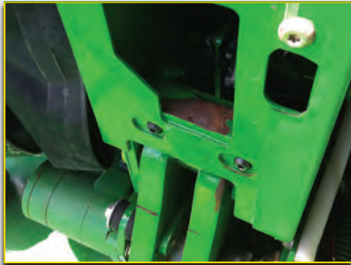
B. Clean the gate latch sensor area.
