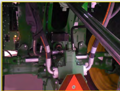
B. Clean the rear axle U-joints, tie rods, motor, and hoses.
