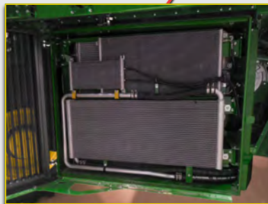
C. Open cooling module door. Clean the door and door latch.
