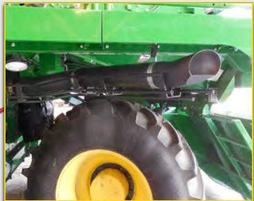
E. Clean exhaust system components, including heat shields and hanger brackets.
