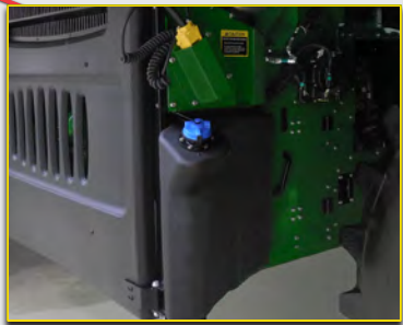
F. Clean the diesel exhaust fluid (DEF) tank and pump (if equipped). Clean access panel latches.
