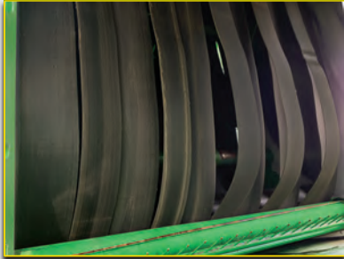
A. With the rockshaft raised, clean and check the belts and rollers inside RMB.
