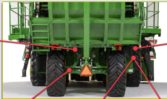
E. Clean the alternators and check the engine belts and pulleys.
