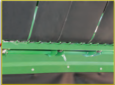
C. Clean and check the wrap feed rods. Clean out debris around the lower gate roller.
