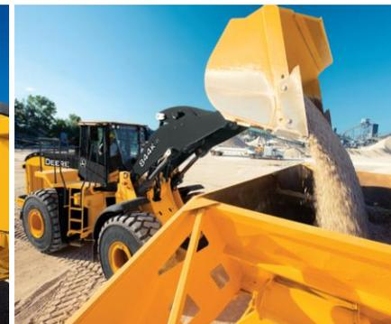
Boom-height kick-out sets maximum desired dump height, while return-to-carry determines lowered-boom position. Use these two K-Series advantages to speed production in repetitive loading applications.
