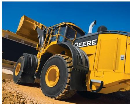
Programmable clutch cutoff increases productivity in all kinds of conditions. Engaging the brakes disconnects the transmission while maintaining high engine speed. For smooth dumps, fast cycles, and no machine rollback.
