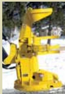
The FS20 is unmatched for high accumulation. The single accumulator arm and two-tined harvesting arm quickly gather large bunches in the big side pocket. The FS20's wide throat opening allows fast, accurate positioning and there's no side discharge assembly to interfere. The side pocket design leaves a wide-open view of the cutting area down to the ground, so the operator's view for felling is unobstructed down to the last tree in the cycle.
