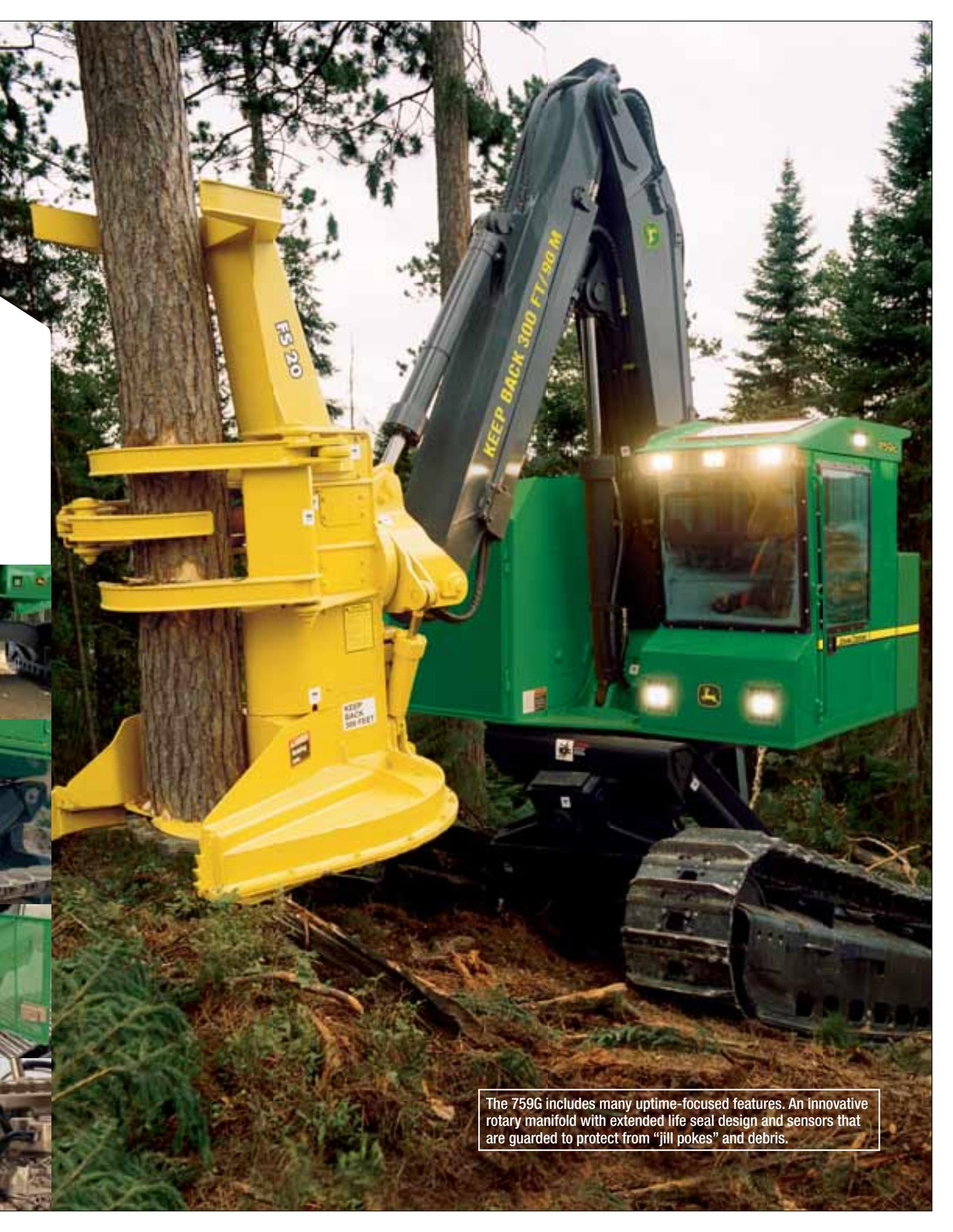
The 759G includes many uptime-focused features. An innovative rotary manifold with extended life seal design and sensors that are guarded to protect from “jill pokes” and debris.
