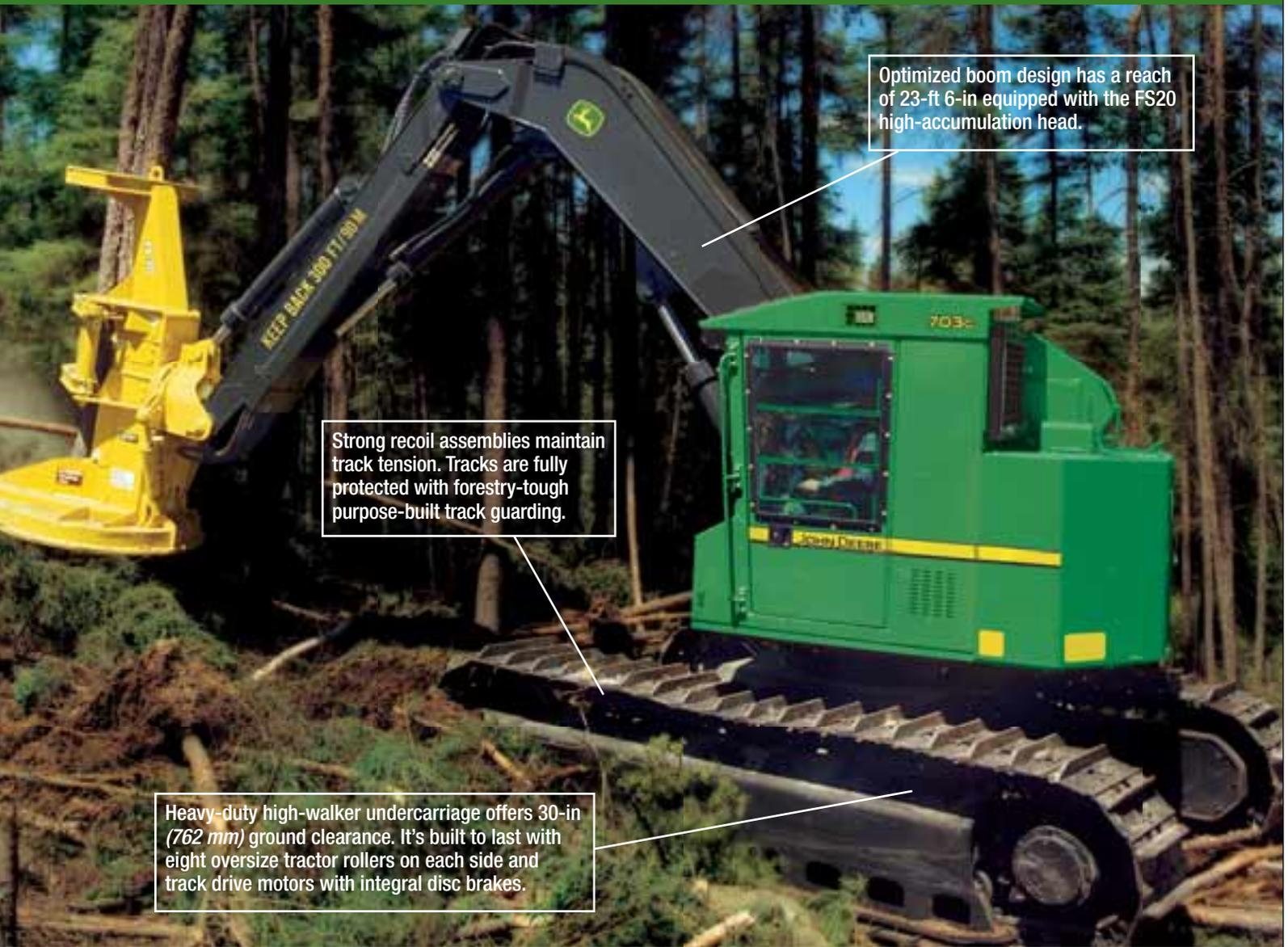
Optimized boom design has a reach of 23-ft 6-in equipped with the FS20 high-accumulation head.
