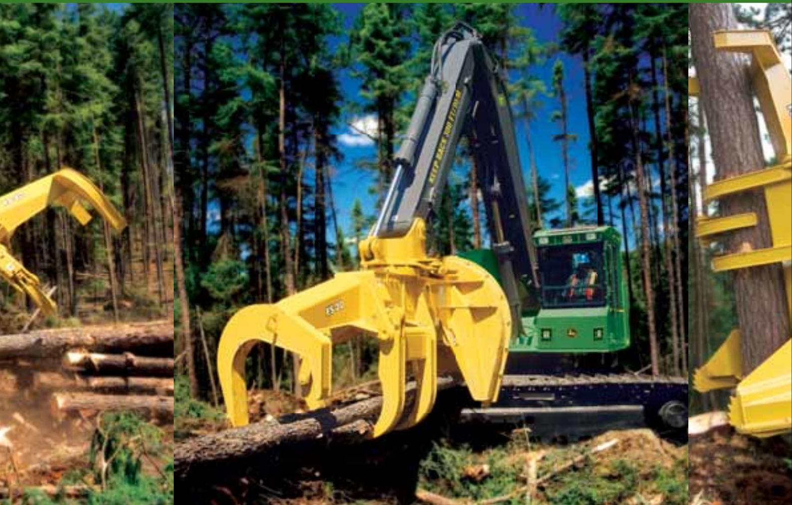
With its large footprint and low center of gravity, the 753G offers incredible stability and low ground pressure from “roll-up.”
