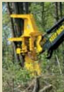
With its center pocket and massively tall single tower and horn, the FS22 gives the greatest control of tall, heavy trees. Two fully synchronized, non-folding harvesting arms and two folding accumulating arms hold larger trees firmly in place. All this means more control of the load and less breakage of valuable harvests.
