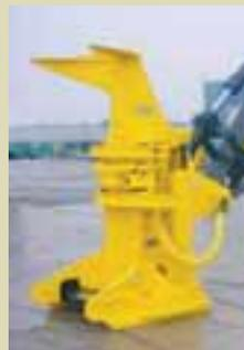
The FG18 high-rotation disc saw has a full 220-degree rotation. Available only with the optional long-reach boom, it allows the operator to cut more wood from one position and use the rotation to stack bigger bunches from two cutting paths into one skidder trail. This allows the skidder to take a full load from one bunch instead of two or three smaller bunches for faster cycle times with less ground disturbance.
