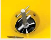
A standard fixed agitator helps material flow through the hopper quickly and easily, and without clogging.
