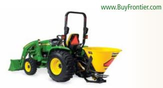
The Frontier Broadcast Spreader is compatible with 20- to 60-horsepower (PTO) tractors and is operated by your tractor's rear 540-rpm PTO.
