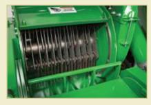
Aggressive 21-inch-wide PTO-driven hammer mill consists of sixty-six, four-way reversible hammers that cut grain consistently. Each durable hammer is made of steel alloy for longer life and repeatable performance. A quick-release pin disengages the mill for mixing-only applications.
