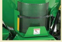
Hammer mill screens are available in a wide range of sizes to vary the consistency of your cut grains. To ensure a uniform mix, a suction fan pulls the ground feed through the screen.
