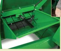
reatures an easy-to-use sack cutter for opening supplement bags, saving you time and reducing spillage. Add minerals directly into the hopper to mix with your grains and create the correct ration
