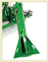
A hydraulic cylinder and motor control the unloading auger from the tractor's operator station. A 300-degree rotation and 53-degree elevation provide remarkable range and maneuverability. An adjustable slip clutch for the unloading auger rotation provides protection against impact (above left).
