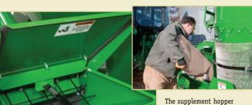
A sliding door controls grain flow to the discharge auger. With this feature, you can control the flow of material into the auger. Closing the door allows for auger cleanout and prevents wasted feed.
