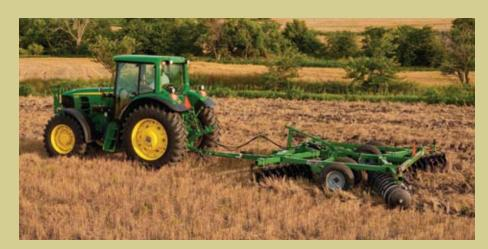
The DH16 Series cuts through heavy corn stalk, thick wheat stubble, tough sod, and more. Adjustable front and rear gang angles let you bury the amount of surface residue to meet your needs.
