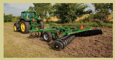
You know you're working with heavy-duty machinery when you hook up a Frontier DH16 Series disk to your tractor. A sturdy frame, 22-inch-diameter and .177 inch thick steel blades, and a commanding 130 pounds of weight-per-blade provide excellent penetration in heavy residue and hard ground.
