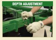
A convenient adjustment pin lets you set depth, fast and easy, and maintains that depth on every pass – so you don't have to worry about cylinder donuts.
