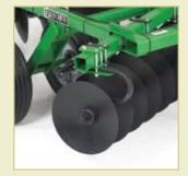
Got rocky fields? The DH16 Series can also be equipped with optional C-spring gang hangers to lessen the shock load and optional .236 inch blades for greater durability when working over rocks and debris.
