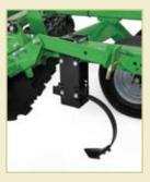
The middle buster (optional) cuts out center balk, and provides a more level soil profile – a key feature to have during seedbed prep.
