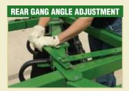
For lighter soils and low residue levels, simply reduce the angle to turnout picture-perfect seedbeds.
