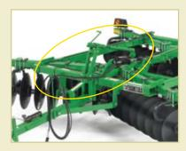
A level-lift hitch provides more-consistent tillage depth when working uneven terrain, and keeps the disk level when making minor depth adjustments, or when raising the machine out of the ground during transport.
