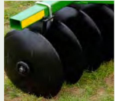
Choose notched or smooth blades with cast spools. Notched blades aggressively cut and mulch, while smooth blades slice and mix residue for a smoother finish. Also choose 7.5-inch or 9-inch spacing on both gangs, or 9-inch on front and 7.5-inch on back.
