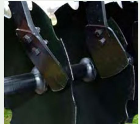
Adjustable blade scrapers are optional on all machines and keep you working in wet, sticky soil.
