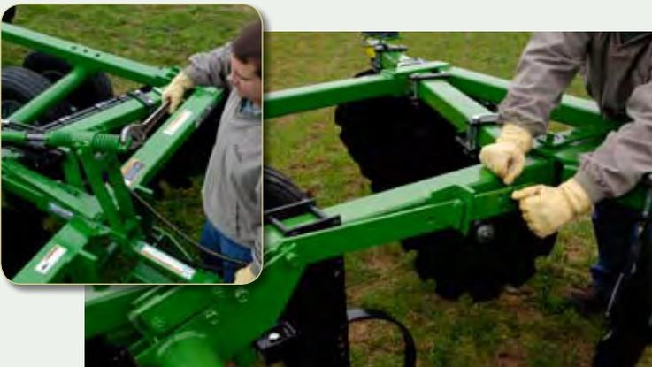
Crank-adjust front-to-rear leveling (left) lets you easily fine-tune disk leveling to avoid ridges and valleys in varying soil types and field conditions. Working depth is controlled with the depth-control bar (right). Simply position the pin and lock it into one of seven positions for the working depth you require.
