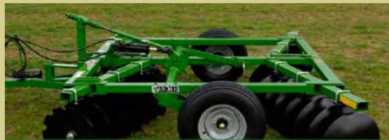
**Frontier DH1510 Disk** – for tractors with 45 to 75 horsepower – handles tough residue with ease. Its rugged construction and wider working width makes it ideal for moderate-sized fields. Choose from smooth or notched blades on 7.5-inch or 9-inch spacing. Working width is 10 feet 6 inches. (Shown with notched and smooth blades.)
