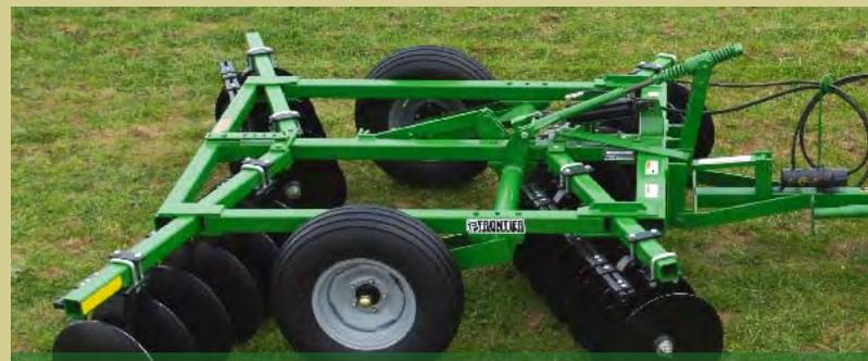
**Frontier DH1509 Disk** – for tractors with 40 to 65 horsepower – features the same rugged construction as the DH1508, but in a larger size. Choose from smooth or notched blades on 7.5-inch or 9-inch spacing. Working width is 9 feet 6 inches. (Shown with smooth blades and optional blade scrapers.)
