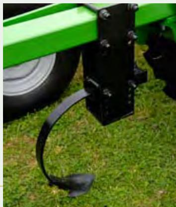
The middle breaker cuts out the center balk for a more level soil profile, ensuring complete coverage on each pass.
