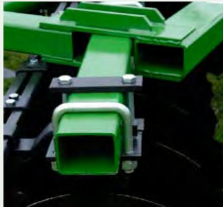
The rugged, heavy-duty tubular steel frame keeps the disk running smooth and level.
