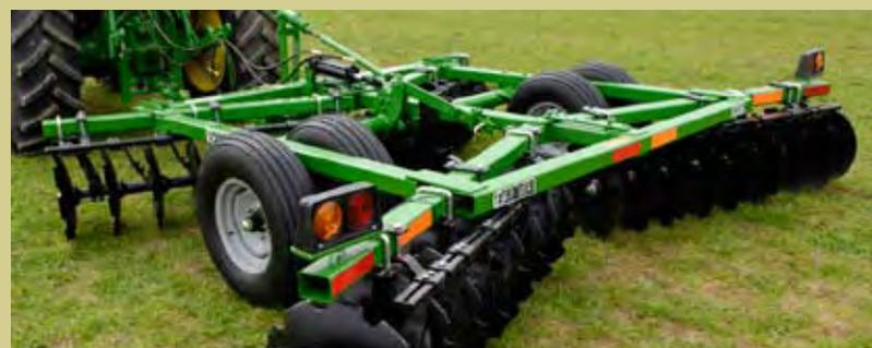
**Frontier DH1512 Disk** – for tractors with 55 to 80 horsepower – is the largest of the DH15 Series Disks. It's built to handle thick residue and tough field conditions. Choose from smooth or notched blades on 7.5-inch or 9-inch spacing. Working width is 12 feet. (Shown with notched blades, standard transport lights, optional furrow fillers, optional middle breaker, optional blade scrapers, and optional dual tires.)
