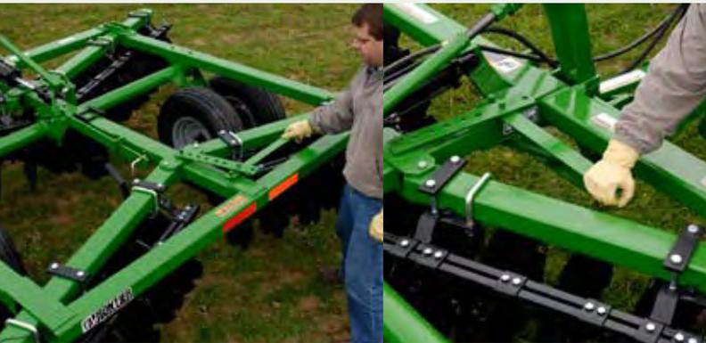
Gang angle adjustments are fast and easy. Just remove the locking pin and slide the gangs to one of nine settings.
