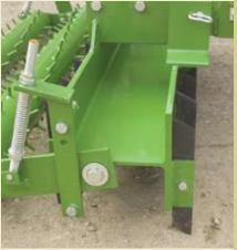
The steel rollers studded with 3/8x1-inch spikes follow the teeth to break down clods. Two, 160-pound compression springs keep the roller in contact with the ground and force the spikes into the soil down to an inch deep. Add an optional second roller with two, 80-pound compression springs for an even smoother finish.
