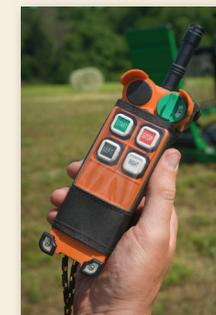
The convenient remote steering and shutdown controller makes wrapping bales a true one-man operation. It allows you to manage the functions of the bale wrapper's operator box from up to 100 feet, so you can sit comfortably in your tractor seat, prepping more bales for rapping.
