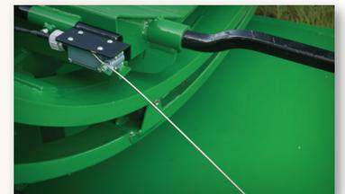
A durable roller bed lets you push off bales fast and easy (top middle and right). And a quick-start rear deck (LW1166 only) helps you create a line of bales with no air pockets, reducing hay spoilage. Guide rollers (standard on LW1166; optional on LW1266) keep each bale centered on the roller bed when wrapping on a slope.
