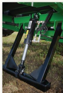
On the LW1266 model, the optional power jack keeps the bed level to start wrapping, preventing air pockets in the line. It then lowers the rear bed to the ground for continuous wrapping as each bale is pushed off.
