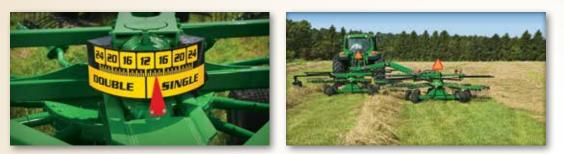
One windrow or two? The RR2324 Tandem makes the decision simple. Just choose the double- or single-windrow option to adjust the twin rotors, and then set the desired windrow width.
