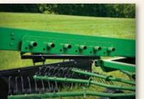
Frontier Rotary Rakes feature cam-action tine arms (bottom-left) that help to gently deposit material into the windrow, while retaining valuable crop. The cam-action movement allows the tine arms to form higher, fluffier windrows that increase drydown. Tine arms can be manually detached (bottom-right) and positioned upright for easy transport and convenient storage (top).
