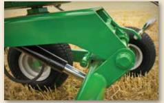
The RR2109, features a rear height-adjustment screw that lets you set the height of the tines for optimal performance in a variety of crop conditions.
