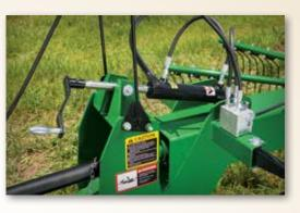
Use the rake-leveling cylinder to set the rake's tine height and pitch. This adjustment allows you to fine-tune ground-pressure in a variety of crops and conditions.
