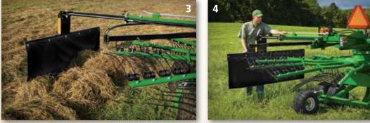
(1) An adjustable, heavy-duty vinyl curtain on the RR2109 and RR2211 helps maintain consistent windrow width. Remove the curtain to combine multiple windrows. (2) An easy-to-use hand lever on the RR23 Series offers fast, simple control of windrow width. (3) When using the RR2324 Tandem Rotary Rake, the rear curtain can be adjusted hydraulically to vary windrow width. (4) And the rear curtain on the RR2324 can also be adjusted with a pull of a lever for quicker transport.
