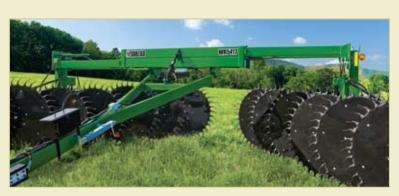
The WR5417 offers a maximum raking width of 29 feet for wider coverage. Or if your operation calls for one-sided raking, the rake wheel beams can be angled independently to the desired position. Hydraulically adjust your windrow width from 24 inches to 72 inches from the seat of your tractor.
