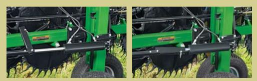
The rake beams on the WR5417 can be locked for easy transport and storage.
