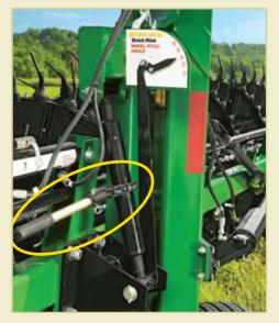
The rake beams on the Frontier Heavy-Duty Wheel Rake feature variable adjustment for setting the wheel straight or tilted based on an 8-degree of difference. Decrease angle to minimize debris pickup, or increase angle when gathering wet hay. Use the ratchet handle (*highlighted*) to adjust tilt angle. The handy meter lets you know when you're at your desired angle.
