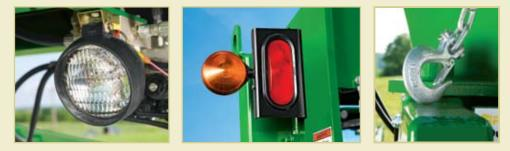
A convenient work light *(left)* helps keep you working safely and efficiently at night. Road lights *(center)* come standard. Beam locking chains *(right)* are also standard equipment.
