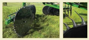
When working in gusty conditions or light hay, the wind panels *(left)* minimize crop loss through the rake wheels, and prevent hay from wrapping around the wheel hub. 60-inch rake wheels help to increase efficiency, and rubber-mounted teeth *(right)* are designed to handle your crop with care.
