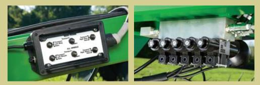
Make a variety of rake adjustments – like windrow or transport width – all from your tractor seat by using just one hydraulic remote (*not shown*) to activate the switches on the rake's electric control box (*left*). The control box connects to the rake's hydraulic valve bank to activate all of the cylinders (*right*).
