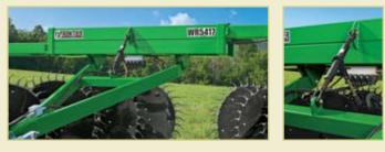
An easy-to-turn ratchet (*right*) enables you to adjust the mainframe so that the rake's beams stay horizontal to the ground for uniform raking.
