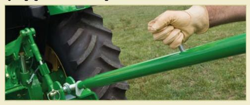
Set cutter depth with the manual turnbuckle adjustment. Shorten the turnbuckle to reduce cutting height. Or for higher cutting height, increase turnbuckle length.
