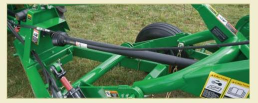
Hydraulic lift rockshaft lets you lower and raise your disc mower from the tractor seat. Transport lock-up bracket prevents your disc mower from lowering during transport, avoiding potential damage to the implement.
