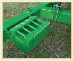
Mounting brackets let you add weights on the caddy to provide additional ballasting when working with larger disc mowers.
