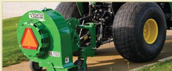
Frontier BL1130 3-Point Debris Blower is compatible with the iMatch Category 1 & 2 quick-attach hitch systems. iMatch converts your tractor's 3-point hitch to fixed attachment points for quick and easy connection. (*iMatch sold separately.*)
