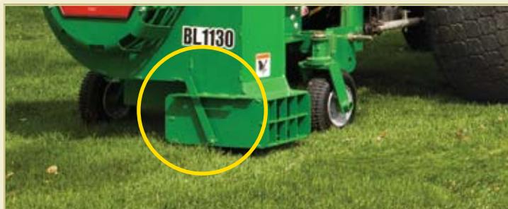
Use this handy adjusting lever (*highlighted*) to change left-right position of the discharge outlet.
