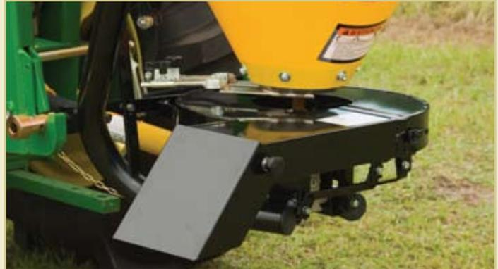
The siderow discharge deflector (*optional*) is easily adjusted to give you improved accuracy and control during discharge.
