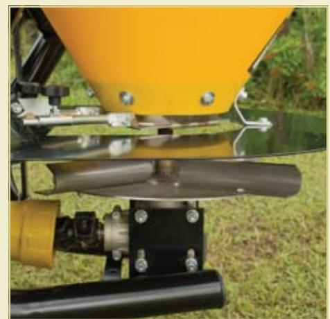
Adjustable stainless steel fins let you change the spread pattern from left to right to center to control your distribution pattern. And the rugged, corrosion-resistant spreading disc helps protect and extend the life of the fins.
