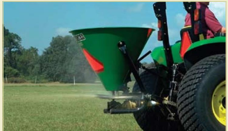
With the **PTO-Driven** Broadcast Spreader, you can spread seed, granular fertilizers, crystalline herbicide, pesticide, sand, and salt at 540 RPM's and in three diverse patterns. Each unit features heat-treated paint to prevent corrosion, and comes standard with a fixed agitator and shielded driveline gearbox.
