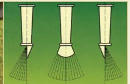
Rotate the optional multi-directional tip left, right, or center for different spread positions. Ideal for spreading near walls or fences, the tip can be placed upright, allowing for close-distance discharge.
