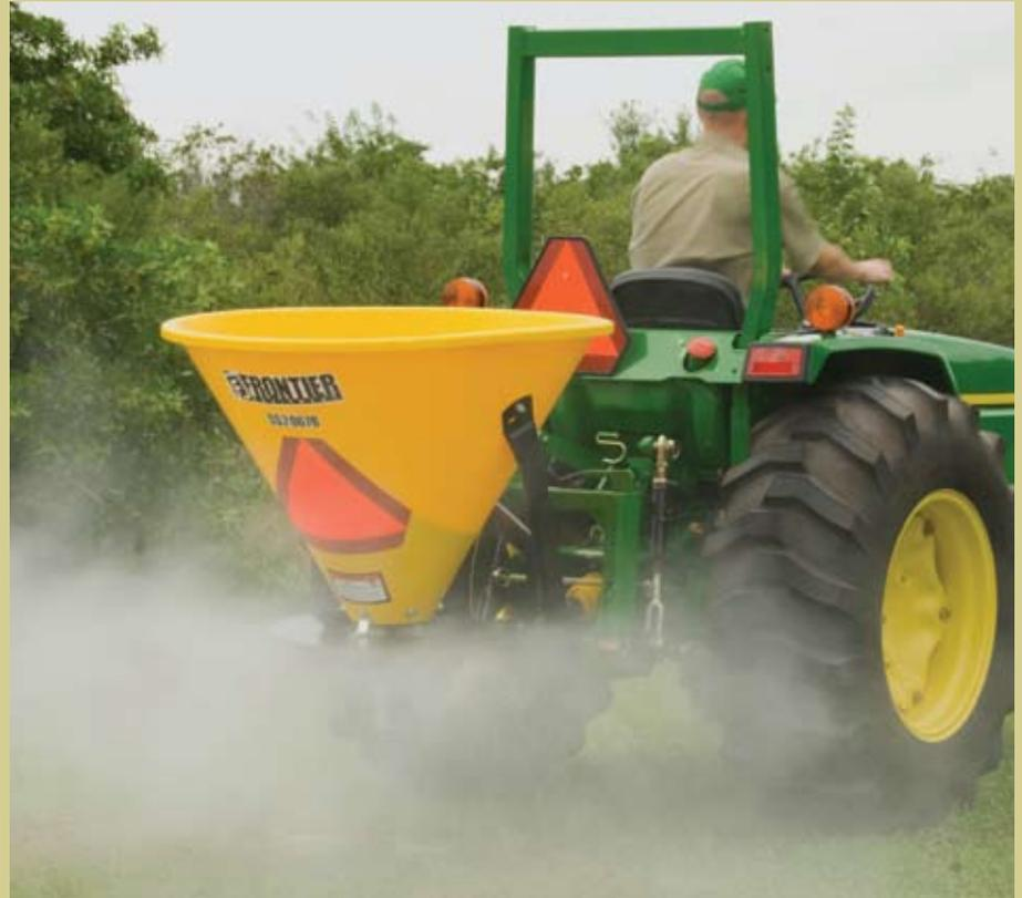
Frontier Broadcast Spreaders are available in two affordable lineups – the steel-hopper 10 Series and the polyethylene-hopper 20 Series. With a capacity range of 3.5 to 10.6 cubic feet and a spread distance of 20 to 46 feet, you get reliable, versatile performance to meet all your spreading needs.
