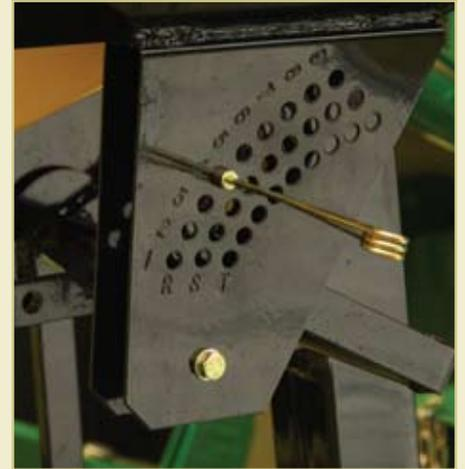
Make simple adjustments to your discharge rate by changing the settings on the spreader rate control. Move the pin higher to increase flow rate or lower to decrease flow rate.
