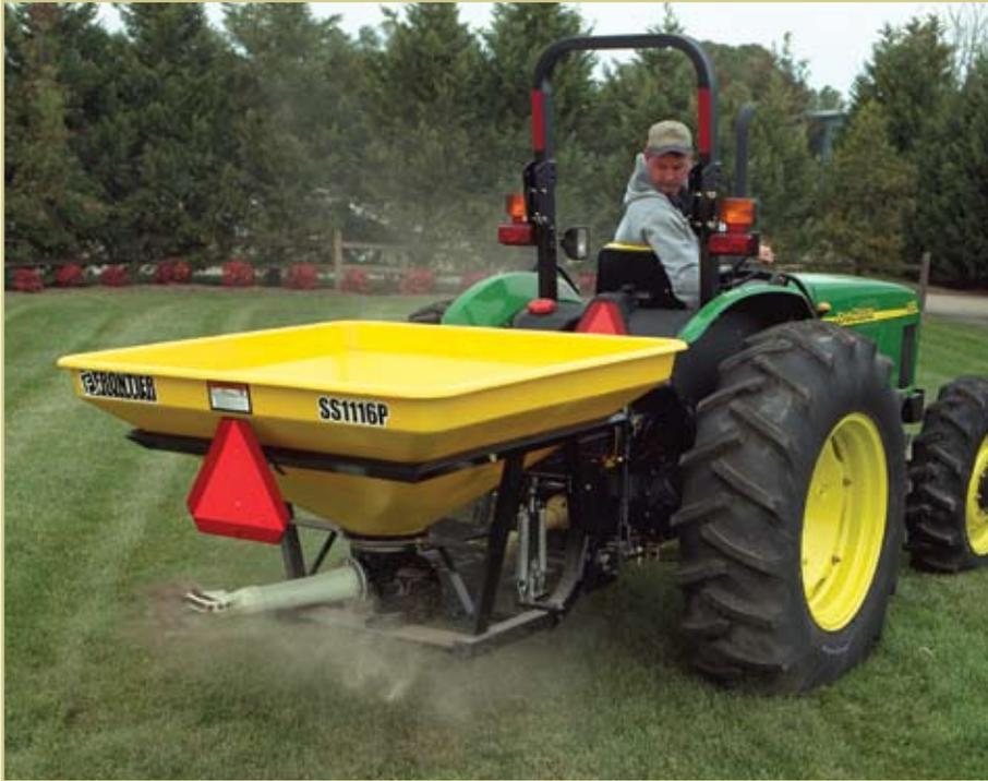
The **Frontier Pendular Spreaders** are equipped with reinforced fiberglass hoppers and stainless steel spreading components. Plus, the heavy-duty drive system is oil-bath lubricated for longer life.
