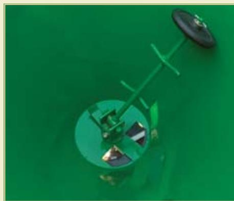
Optional wheel agitator keeps material from packing and bridging over the discharge.
