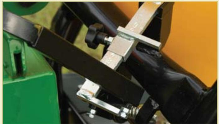
The feed rate lever is conveniently operated from the driver's seat to open the spreader gate when dropping seed and fertilizer.
