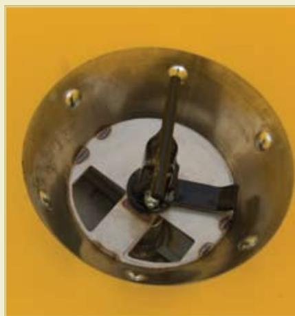
Standard agitator helps prevent clogging in the hopper when using powdered or high moisture fertilizer. The durable hopper gate is stainless steel to avoid corrosion.
