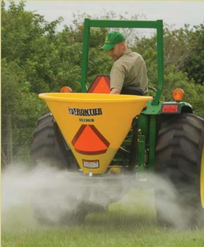
The **20 Series Broadcast Spreaders** feature a polyethylene hopper and stainless steel spreading components for strong resistance to salt, sand, and other corrosive material. This helps prevent rust and weather damage to minimize maintenance and extend spreader life.
