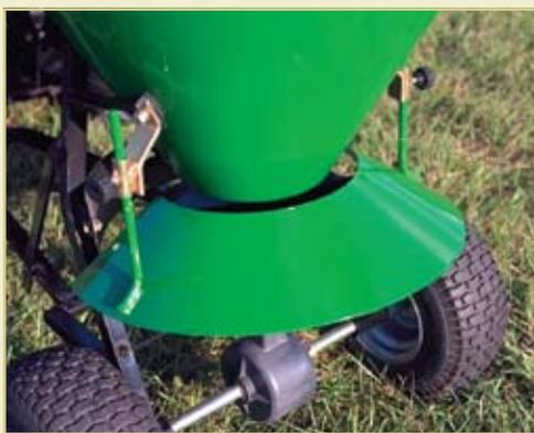
A rugged deflector shield (*optional*) helps ensure uniform spread swath and keeps salt on your sidewalk.
