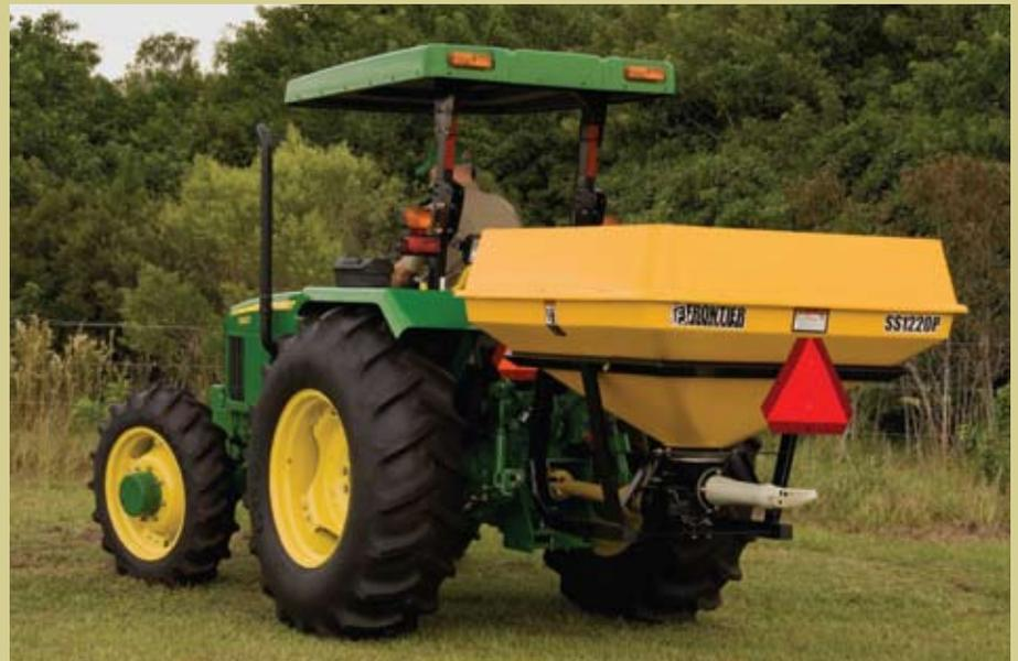
Pendular Spreaders come in four high-performing models to handle commercial jobs. Ranging from 792 to 2,205 pounds of capacity and offering an accurate 17- to 46-foot spread, Pendular Spreaders allow you to cover more ground in less time.
