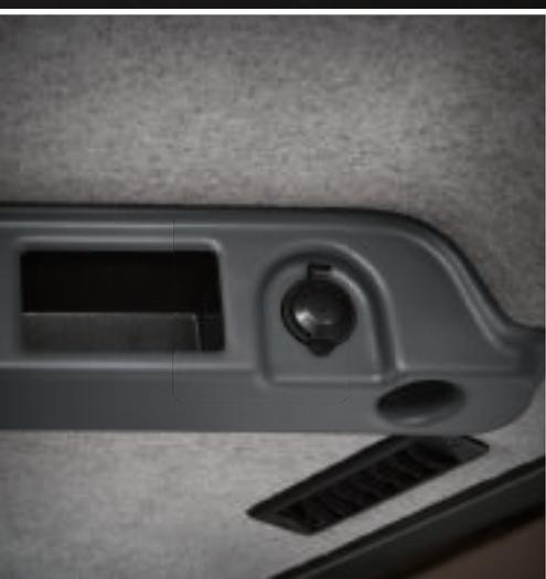
1. Sealed-switch module allows low-effort control of keyless start, and enables exclusive features such as turbocharger cool-down and auto shutdown. Touchpad security system requires a numeric pass code (when enabled) to help prevent unauthorized machine operation.
