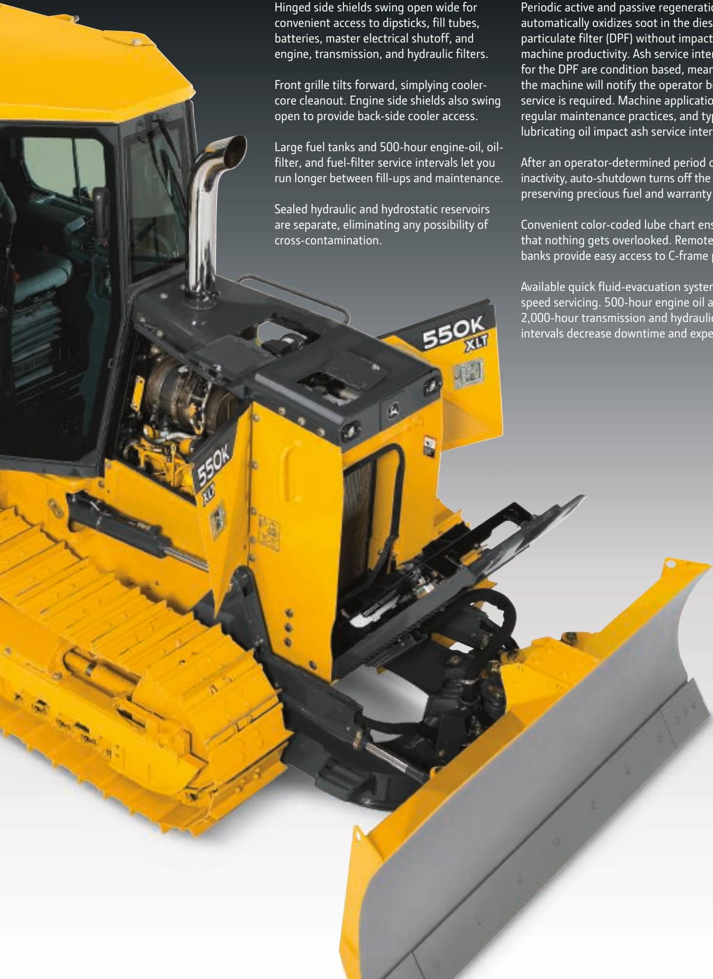
Hinged side shields swing open wide for convenient access to dipsticks, fill tubes, batteries, master electrical shutoff, and engine, transmission, and hydraulic filters.
