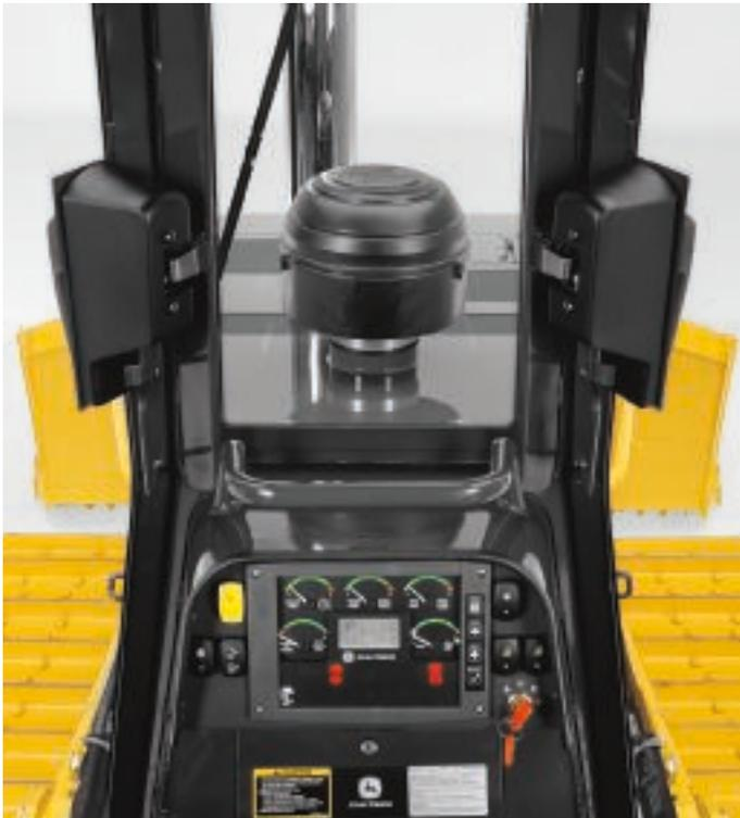
Cab-forward design positions the operator for a more stable ride and a commanding view behind, below, and beyond the blade. Side and rear visibility is equally unobstructed. Monitor keeps a vigilant watch on vital machine functions with warnings you can see and hear.
