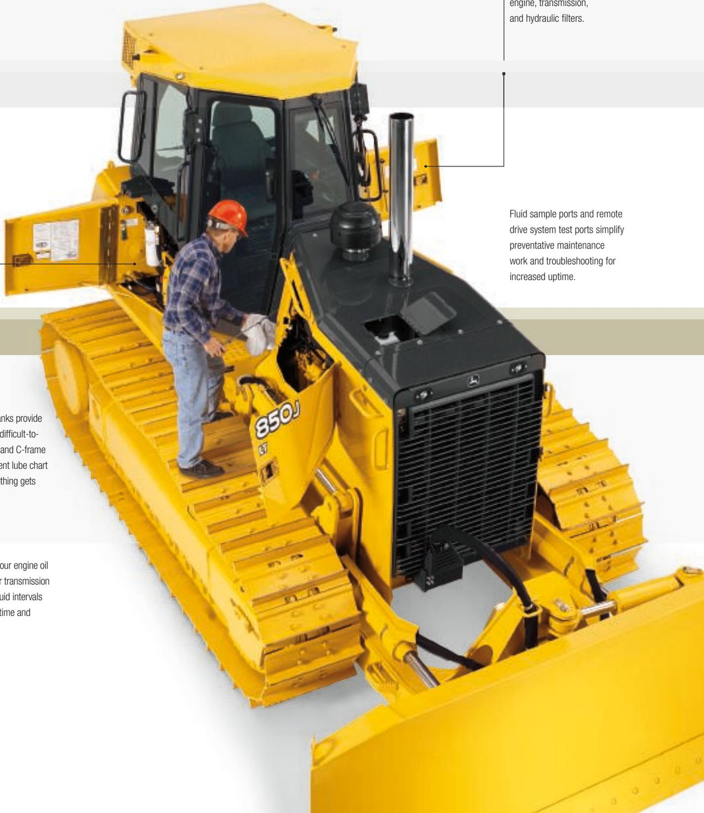
Fluid sample ports and remote drive system test ports simplify preventative maintenance work and troubleshooting for increased uptime.
