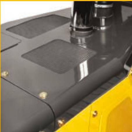
Perforations act as a “first filter,” preventing entry of most debris. Anything that gets past the five-mm holes also easily passes through the cooler cores.
