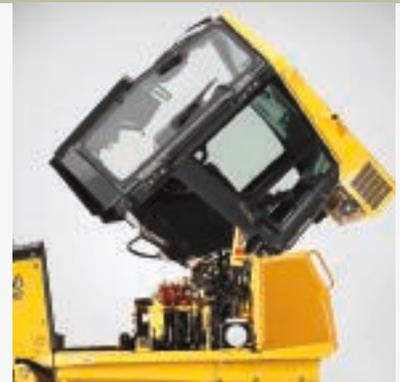
Operator station tilts a full 70 degrees in only minutes, for wide-open access to internal components. Unlike other crawlers, there's no need to disconnect linkages, hydraulics, or wiring.
