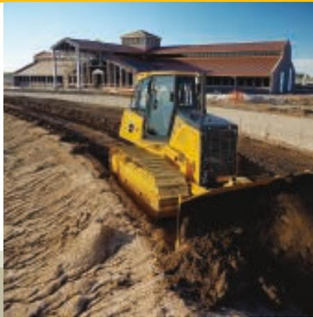
Independent track control speeds up or slows down each side – for smooth, full-power turns. An automatic 10-percent power boost helps carry more material in a turn.
