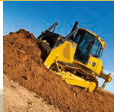
No need to cross-steer or ride a brake. These dozers steer the same and maintain their preset speed whether working on level ground or a 2-to-1 slope.
