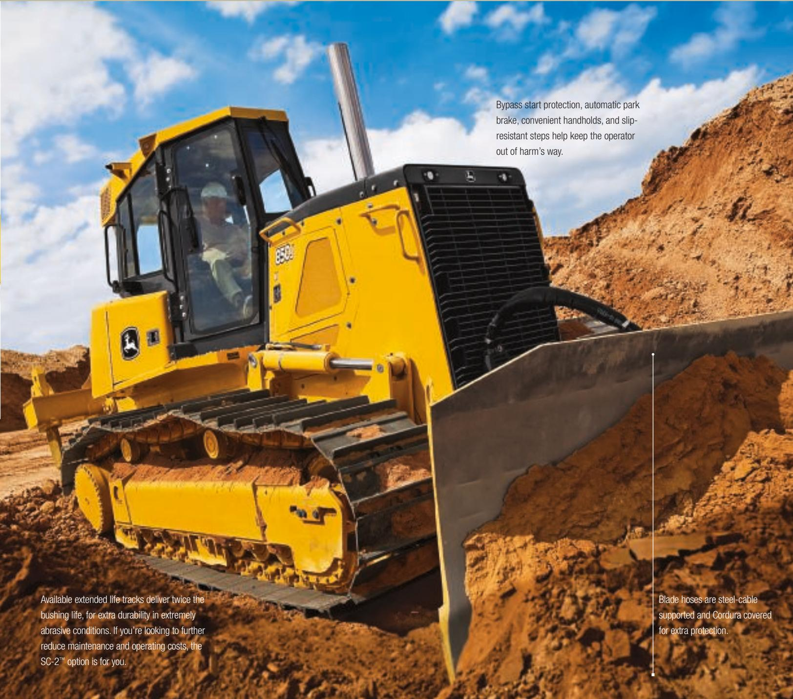
Bypass start protection, automatic park brake, convenient handholds, and slip-resistant steps help keep the operator out of harm's way.
