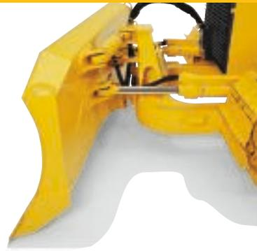
The PAT dozer's closed-cell blade design and box-section C-frame deliver exceptional strength and durability. Outside-mounted dozer push beams are equally durable.
