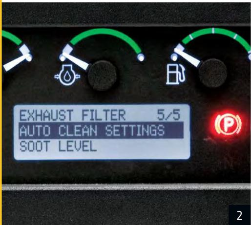
2. Exhaust filter operation and status are indicated with icons and on-screen displays. The diagnostic monitor also provides easy-to-understand messages that help speed troubleshooting.
