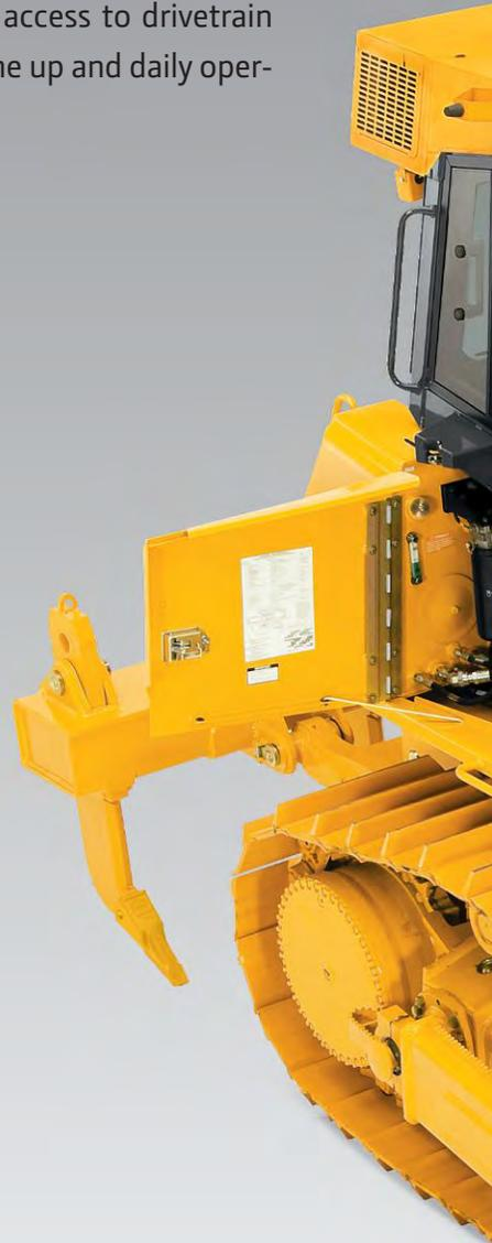
Hinged side shields swing open wide for convenient access to dipsticks; fill tubes; batteries; master electrical shutoff; and engine, transmission, and hydraulic filters.
