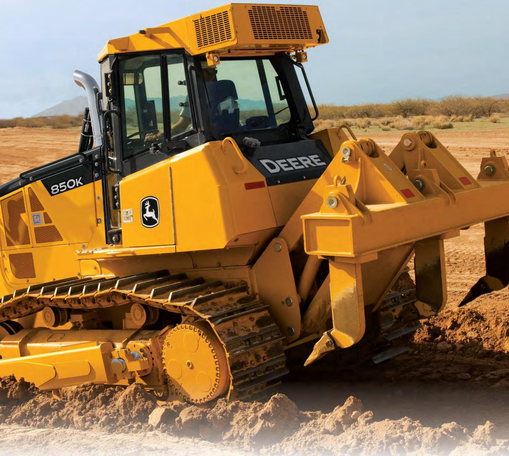
Flush-fit bottom guards and tight-fitting side shields help keep trash out. Hood and side-shield perforations function as a “first filter,” further preventing entry of most debris. Anything that gets past the five-mm holes also passes through the cooler cores.
