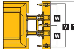
Multi-shank (3) parallelogram ripper with hydraulic pitch adjustment and ESCO® ripper tips
