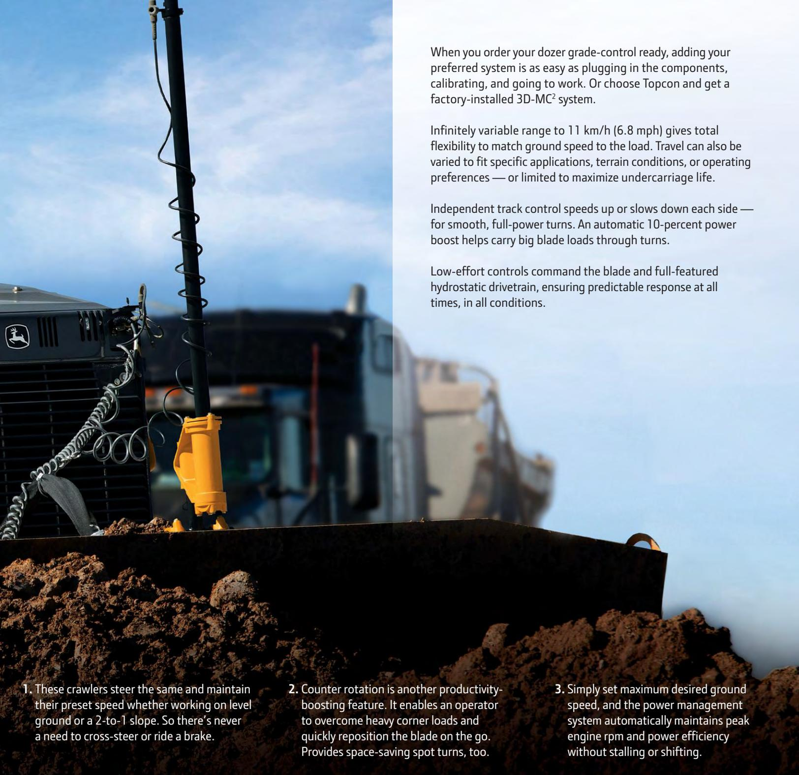
When you order your dozer grade-control ready, adding your preferred system is as easy as plugging in the components, calibrating, and going to work. Or choose Topcon and get a factory-installed 3D-MC<sup>2</sup> system.
