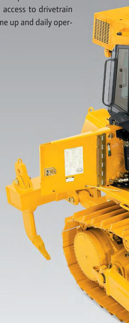
Hinged side shields swing open wide for convenient access to dipsticks; fill tubes; batteries; master electrical shutoff; and engine, transmission, and hydraulic filters.
