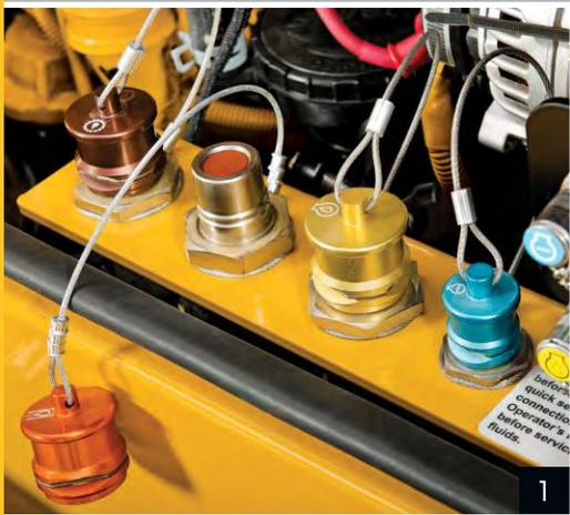
1. Available quick fluid-evacuation system helps speed servicing. 500-hour engine oil and 2,000-hour transmission and hydraulic fluid intervals decrease downtime and expense.
