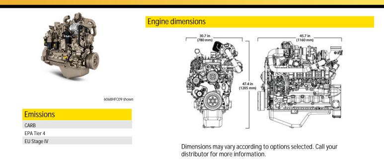
General data Model 6068HFC09 Length - mm (in) 1160 (45.7) Number of cylinders 6 Width - mm (in) 780 (30.7) Displacement - L (cu in) 6.8 (415) Height-- mm (in) 1205 (47.4) Bore and Stroke-- mm (in) 106 x 127 (4.17 x 5.00) Weight, dry - kg (lb) 785 (1731) **Compression Ratio** 16.7:1 Engine Type In-line, 4-cycle Aspiration Turbocharged and air-toair aftercooled
