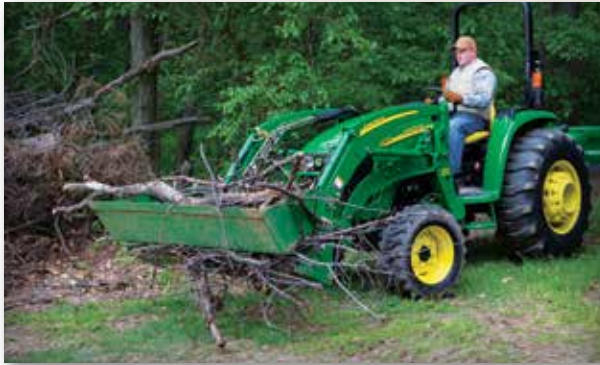
Use the 4-in-1 Bucket to clear logs or debris (left), or use it as a dozer to grade and smooth driveways (right).
