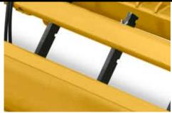
Scarifier height is easily adjustable. Simply remove the shank key and raise or lower the scarifier to one of four settings. Use the top notch for deeper ground penetration.
