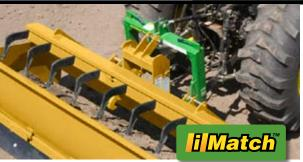
All 41 and 42 Series Hydraulic Box Blades are compatible with the John Deere iMatch™ quick-hitch system. iMatch converts your tractor's 3-point hitch to fixed hooks and attaching points for a super-quick connection. Select models are Category 2 Quick Coupler compatible. (iMatch hitch sold separately.)
