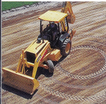
A 50-degree turning angle gives the 310E a tight 11-foot 9-inch turning radius for easy moves in close quarters.
