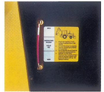
This sight gauge provides a quick, contamination-free check of the hydraulic oil level.
