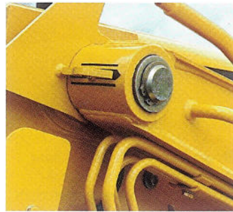
Bucket level indicator is within your line-of-sight. Nearby automatic return-to-dig switch is well-protected, yet easily accessible. Hydraulic self-leveling and float are also standard.
