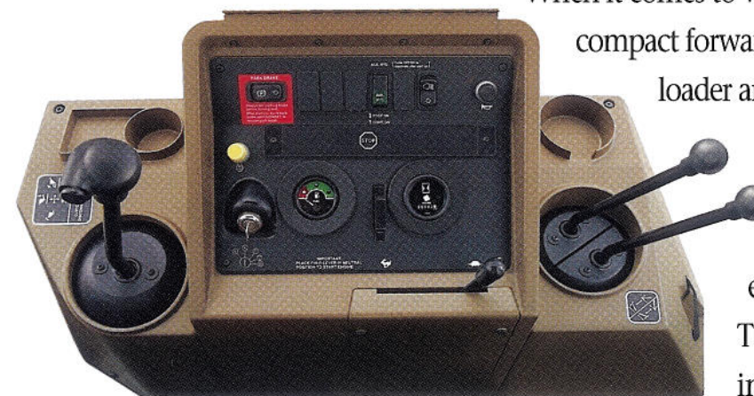
Electronic monitor or optional gauges provide vital machine information at-a-glance from either operating position. Console also houses seat belt warning, ignition and automatic parking brake switches, and climate controls (with cab). Switch for MFWD is conveniently positioned and uniquely shaped for no-look on and off.
