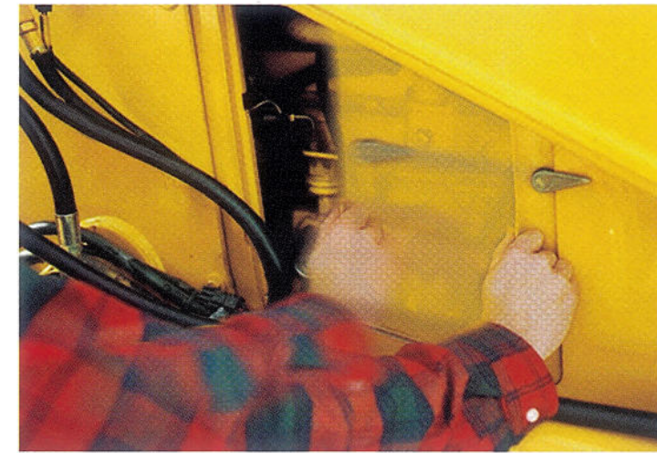
This sight gauge provides a quick, contamination-free check of the hydraulic oil level.
