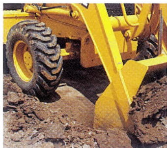
Available mechanical-front-wheel drive provides extra power and traction to keep the bucket heaped regardless of what's underfoot.
