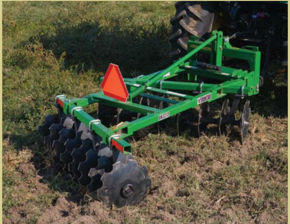
The DH32 Series 3-Point Offset Disks are ideal for small utility tractors from 30 to 75 horsepower, and are available in cutting widths of 5-feet 3-inches to 8-feet 4-inches.
