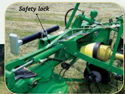
The TD1316 (left) has four rotors. The outer two rotors hydraulically fold up and manually pivot 180 degrees for narrower transport and stability. A safety lock keeps the rotors in place during transport.
