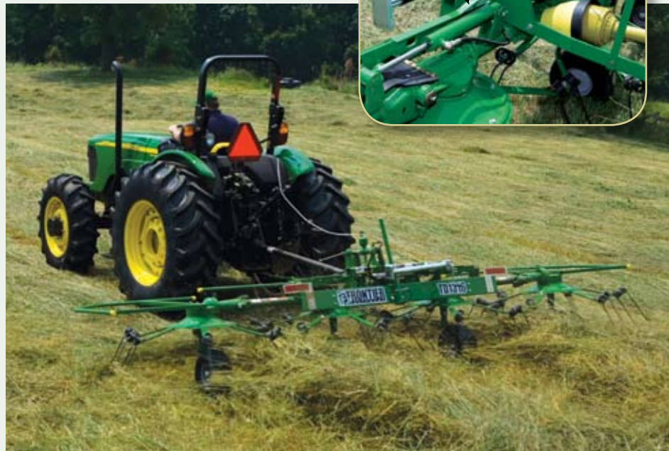
On the TD1316, folding and unfolding of the outer rotors, as well as the release of the transport safety lock, is made from the tractor seat.
