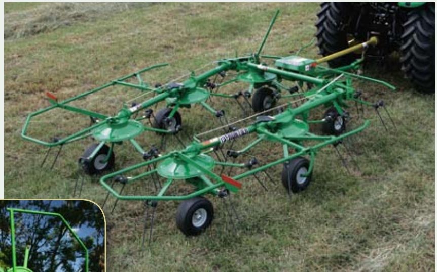
The TD1123 (above) has six rotors. The outer four rotors manually fold to the rear for transport.
