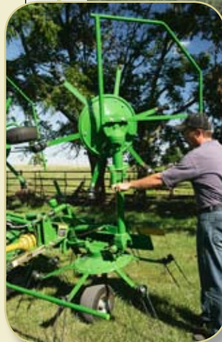
The TD1123 (above) has six rotors. The outer four rotors manually fold to the rear for transport.
