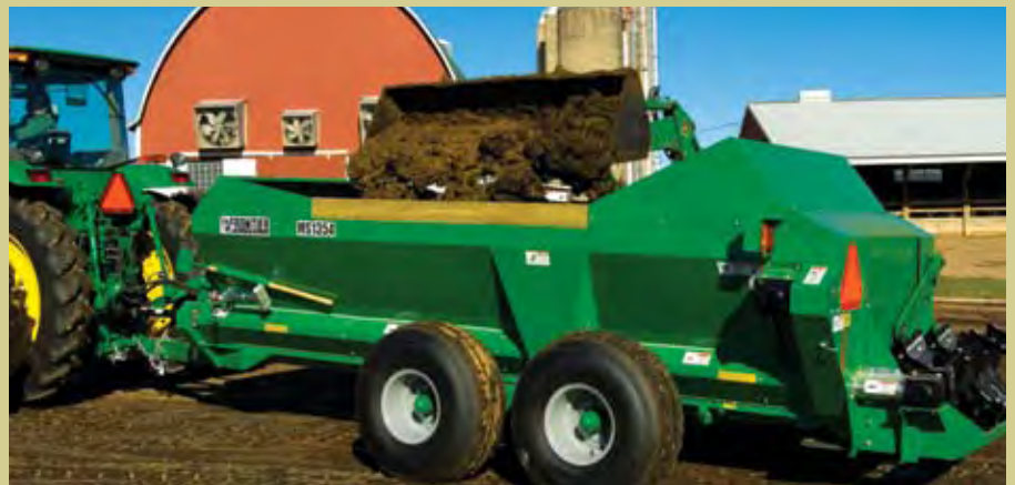
Frontier All-Purpose Manure Spreaders feature a "V" tank made of corrosion-resistant copper-bearing steel. Sides are 1/8-inch thick and ends are 3/16-inch thick. Optional front and rear splashguards help contain the load.
