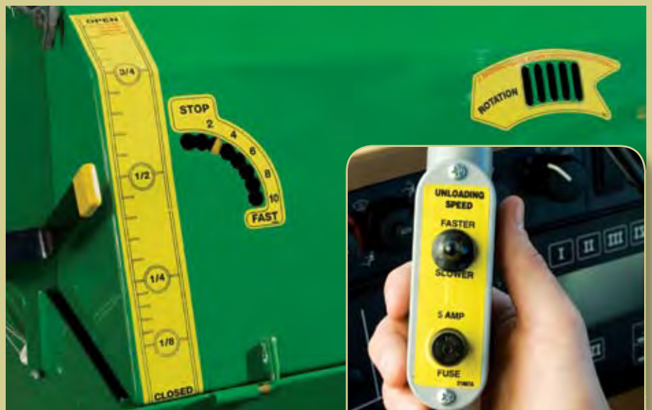
A "dashboard" lets you verify direction of the auger rotation, auger speed, and sequential opening and closing of the endgate and clean-out pan. The dashboard is visible from the tractor cab. A simple variable speed hydraulic drive ( inset ) controls the augers, requires less power, and lets you match the auger feed rate to a wide range of material consistencies. A pressure relief valve protects the drive and augers from overload damage.
