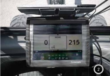
**Measuring and Control System**: Allows the operator to automate the entire tree processing cycle with the touch of a button. Set your log size and length to get the maximum volume and quality out of each and every log.
