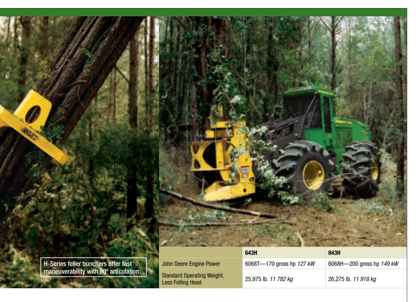
The H-Series feller bunchers are built to be durable with a tapered-roller-bearing center joint and a streamlined hood constructed of dent-resistant steel. Heavy-gauge fuel and hydraulic tanks, as well as the wraparound rear bumper are forest-tough to stand up to the punishment of the woods. They're also built to be more productive with big pins and bushings in the boom and head-tilt linkage to maximize lift capacity.
