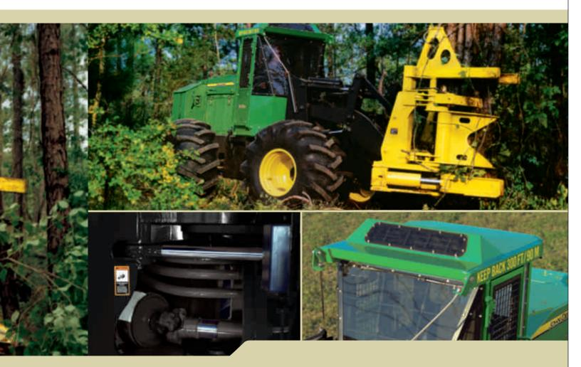
Strong center hinge with large tapered roller bearings give long-life reliability to this critical area.
