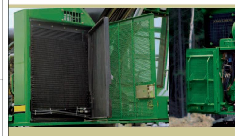
An optional reversible fan purges debris from coolers, which extends the engine's life and makes it run more efficiently.
