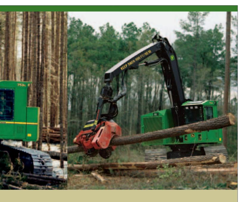
Near-zero tail-swing over the rear with only 10-in. (250 mm) over the side of standard tracks.
