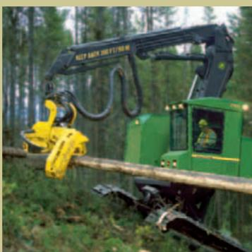
27-in *(685 mm)* saw bar on the 762C automatically extends only far enough to complete the cut, reducing the chance for damage while felling. Powerful feed rollers handle the tree gently, and superior delimbing is handled with four moving and two fixed delimbing knives.
