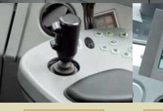
The mini-lever joystick controls mounted on the armrest give you precise control of all loader functions. TMC provides valuable information on the different machine functions, such as average or momentary fuel consumption.
