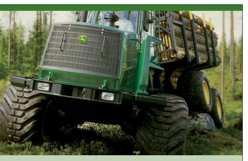
The patented balanced bogie system significantly increases the environmental friendliness of the machine. Evenly distributing the weight between all the wheels reduces the ground impact and provides a smooth ride, even when the forwarder is fully loaded.
