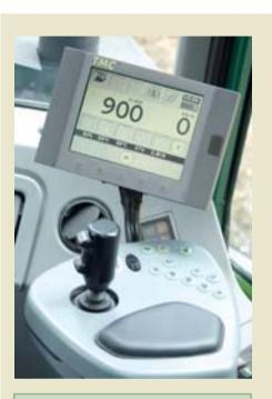
The Timbermatic 700 and the TMC improve overall productivity and allow for easy use of the latest monitoring tools, such as the boom scale and the reverse camera. The sensors and software of the optional boom scale measure the weight of the load and the logs. This allows for efficient use of the load space: the loads remain a suitable size and forwarding is safe and fast. The self-learning calibration function of the scales increases the reliability of the system.
