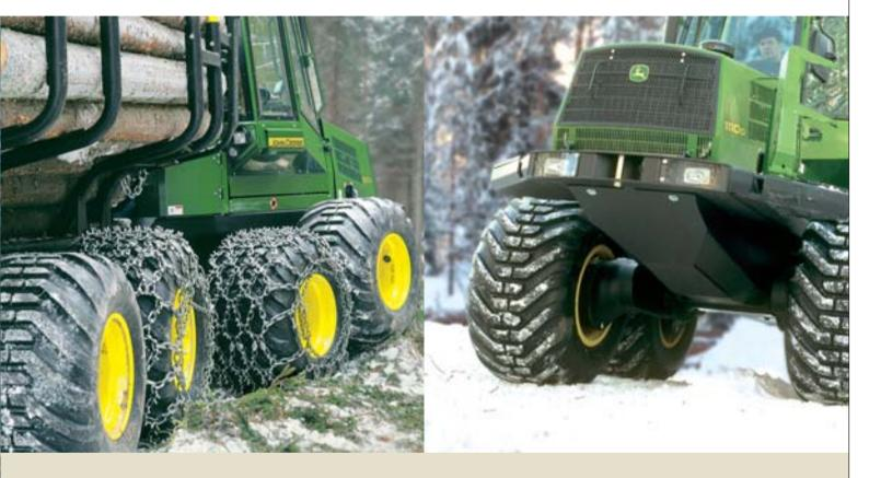
The patented balanced bogie distributes the weight evenly between all wheels. This reduces the ground impact and ensures a gentle ride even when the forwarder is fully loaded. Part of the bogie structure is located inside the rim of the wheel to allow for as high and wide a ground clearance as possible. The machines can thus go over rocks and stumps without difficulties. This helps to choose routes and improves the productivity of the machine.
